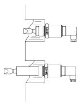
The cable gland should be situated on the lower side of the connector. If it is necessary, the position of the connector can be changed by  $90^{\circ}$  or  $180^{\circ}$ . To do this, open the connector and rotate. This operation must be done with the power disconnected
