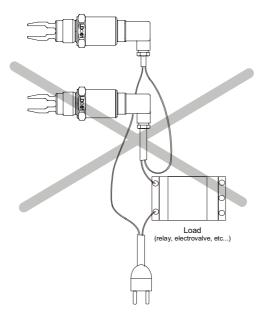
When the LD-61 is connected to detect a maximum level, the load is "activated" when the fork is not in contact with the fluid. In the same way, when the LD-61 is connected to detect a minimum level, the load is "activated" when the fork is in contact with the fluid.
