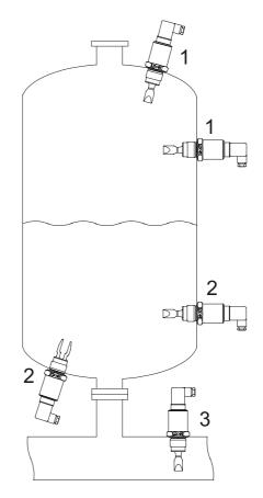
In the same way, when the detector is installed where there is flow, the position must be taken into account. The flat part of the tines must be aligned parallel with the flow direction.
