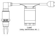
The LD-61 detector cannot be connected in series. Each detector must have its own load.
