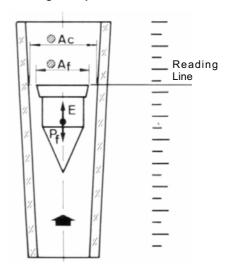
The flowmeter consists of a float inside a conical tube.
