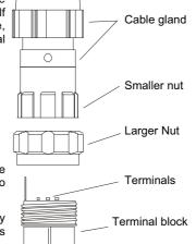
Before making the solder joints, loosen the cable gland nut and pass the cable through it, and also through the larger nut.
