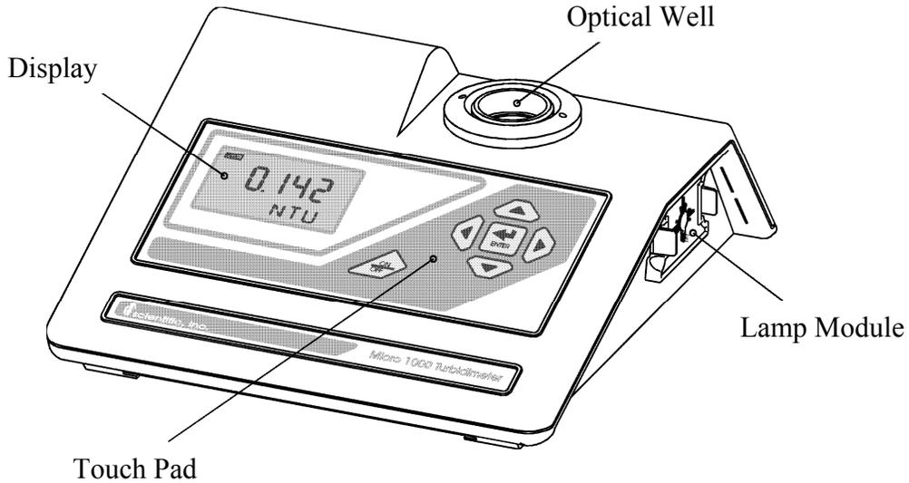
**Figure 1a - Front view of the Instrument**
