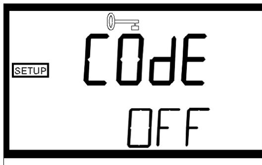
The upper row of the display will indicate the operational status of the security access option (on or off). You can change the operational status of this option using either the ▲ or ▼ keys. Once you have set the desired status, press the
