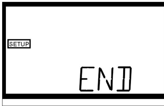
You may also reach this point by pressing either the ◀ or ▶ key until the word “END” appears on the lower row of the display. At this point, simply press the
