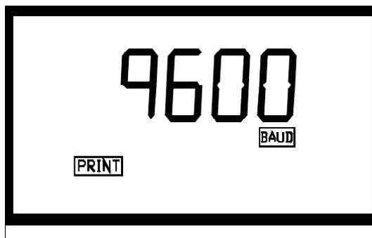
Select the desired baud rate (1200, 2400, 4800, or 9600) by pressing either the ▲ or ▼ keys to change the displayed baud rate. The other RS 232 parameters are fixed at 1 stop bit, 8 data bits and no parity. When you have selected the proper baud rate press the
