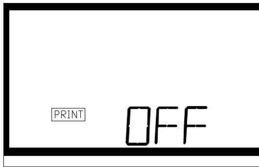
This feature allows you to select the function of the serial port on the instrument. There are two options to choose from: Off and Timed Output. Select the RS232 option by pressing either the ▲ or ▼ keys. When you have selected the proper function, press the
