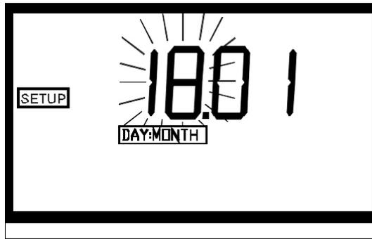
Select the correct day by pressing either the ▲ or ▼ keys to change the displayed day. When you have selected the proper day, press the
