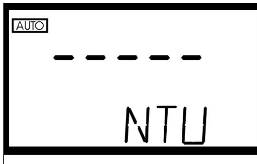
This indicates that either the instrument is performing an auto-ranging function, or the sample has not yet stabilized (e.g. air coming out of solution in the form of bubbles). The dashes should remain for a brief period of time (< 45 seconds). If the dashes remain for an extended period of time please contact the HF scientific, inc. Technical Services Department for further assistance and guidance.
