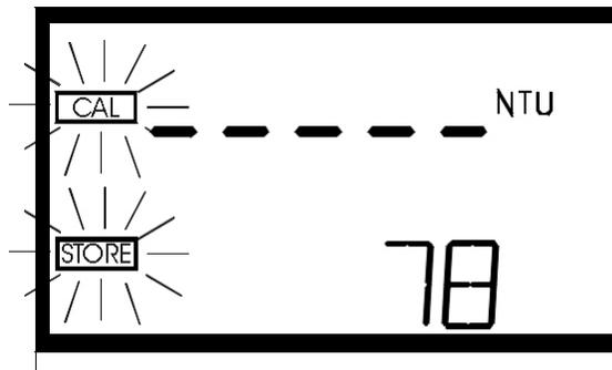
**Note: The 0.02 NTU standard must be evaluated in calibration at both the start and end of calibration to ensure accurate measurements in the ratio mode and when recording FAU measurements.**
