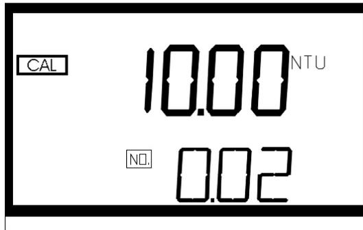
8. Insert the 0.02 NTU calibration standard into the sample well and calibrate as before. When the instrument has completed the calibration, the “Cal” and the “Store” blocks will quit flashing and the lower row of the display should now display the word “END” indicating that the instrument has completed the calibration phase and you can now exit into the normal mode for measurement.
