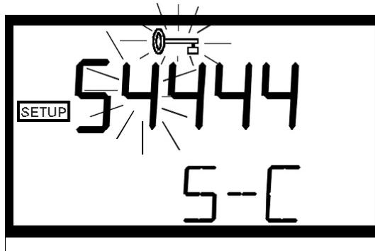
Select the access code for the configuration/setup mode as you did with the calibration mode.
