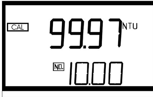
7. Insert the 10.0 NTU calibration standard into the sample well and calibrate as before. When the instrument has completed the calibration, the “Cal” and the “Store” blocks will quit flashing and the lower row of the display should now indicate that the 0.02 NTU standard is the next standard to be used for calibration.
