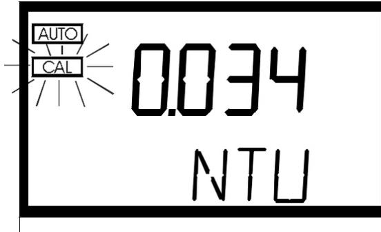
The factory default is 30 days. HF scientific inc. recommends calibration every 30 days. The flashing "Cal" block is only a warning and does not mean that the instrument will stop performing accurately. The "Cal" block will flash until you have re-calibrated the instrument.
