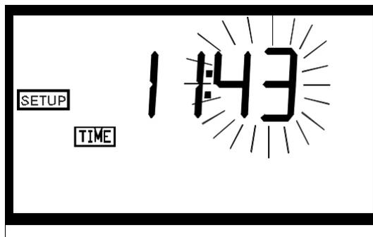
Select the correct minutes level by pressing either the ▲ or ▼ keys to change the displayed minutes. When you have selected the proper minutes level, press the
